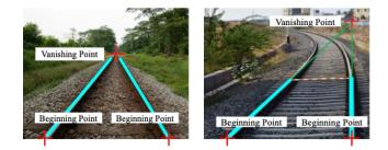
(a) Three points for a Straight Track (b) Three points for a Curve Track
